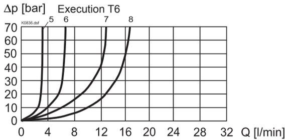
$\Delta p = f(Q)$  Pressure loss/flow characteristics ( $l = l_G$ )
