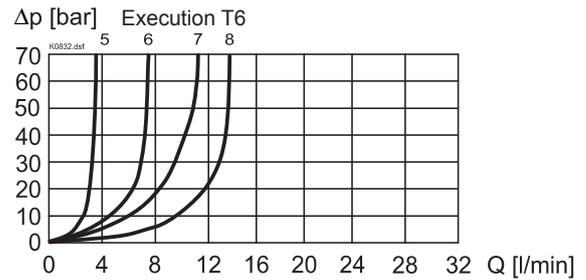
$Q = f(l)$  Volume flow adjustment characteristics ( $\Delta p = 20$  bar)
