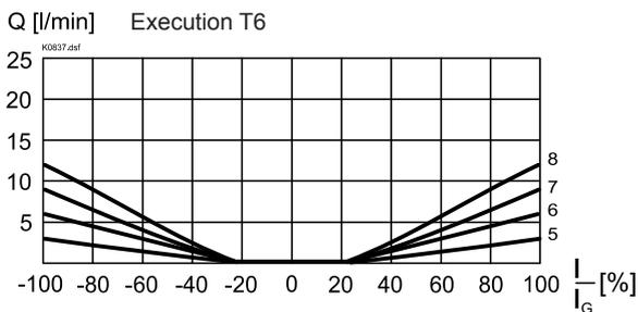
$Q = f(l)$  Volume flow adjustment characteristics ( $\Delta p = 20$  bar)
